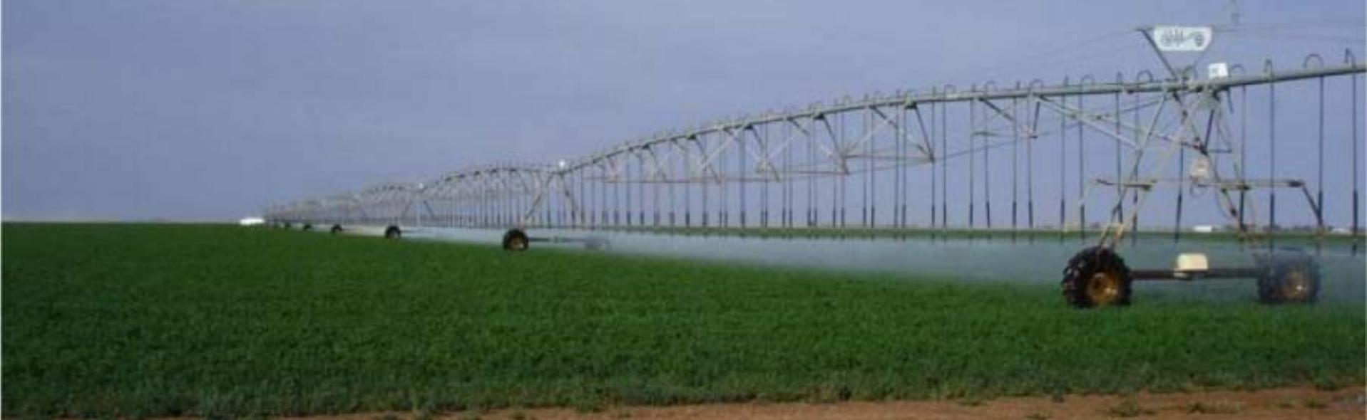
A large center pivot irrigation system is shown over a vast green field. The system consists of a long metal structure supported by many wheels, with multiple parallel pipes extending from a central pivot point. The field is lush green, and the sky is clear blue. The foreground is a dry, brownish soil.
